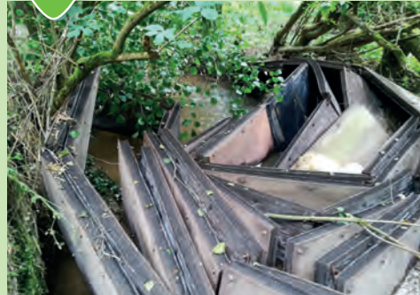
① Example of an experimental floating device installed in an 85m duct carried away by the current, following breakage of the anchorage on the duct head.
