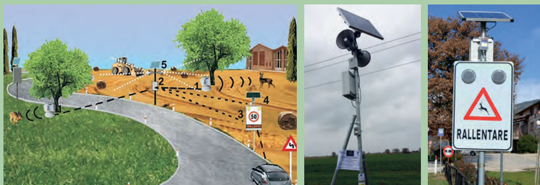
1 Illustration and photos of the alarm/scare system. Source: : http://www.lifestrade.it http://www.lifestrade.it
