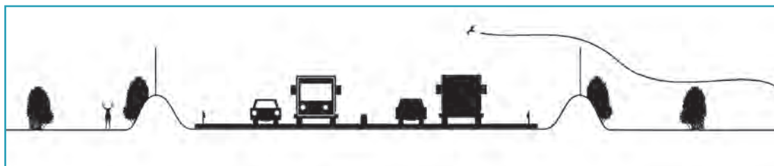
1 Development plan of protective mounds ensuring the protection of flying wildlife and the tranquillity of rights-of-way for terrestrial fauna. Source: Cerema.
