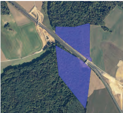
27 Compensatory measure in the surrounding area of the fauna passage. Extension of the A16 motorway on the SANEF network. Source: Geoportail.
