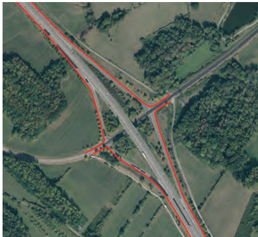
Example the layout of fencing next to an interchange. Source: Google Earth/Cerema.
