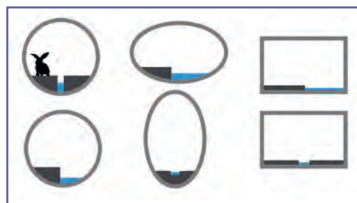
19 Schematic diagram of systems for concentrating low flows in a structure. Source: Cerema.
