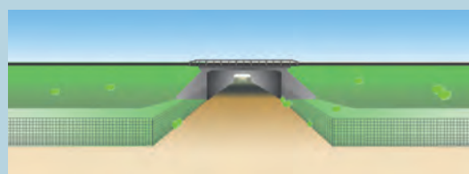
3 The layout of the fencing does not leave the green rights-of-way accessible to wildlife. Its layout near the entrance of the structure creates a corridor effect that deters wildlife. Source: Cerema.
