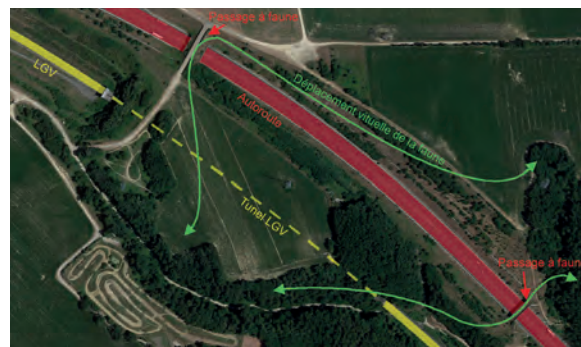
16 Twinned infrastructure where the fauna passages of the road infrastructure are located in continuity with the railway tunnel. Source: Google Earth.
