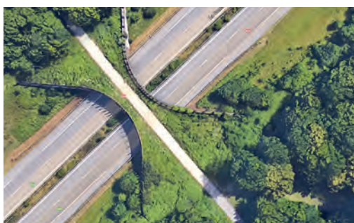
❷ Ordinary mixed all fauna overpass. A36 motorway (Grand Est region). Source: Google Earth.
