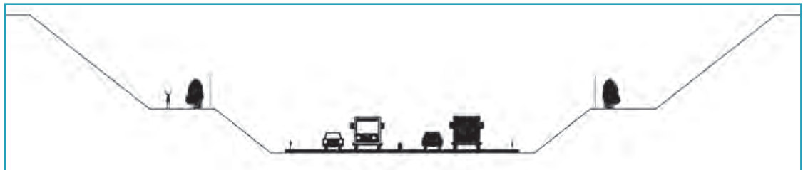
③ Development plan for berms* in large excavation zones to create a zone conducive to the movements of wildlife and to install fencing. Source: Cerema.
