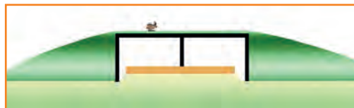
❷ Schematic representation of a structure built on an infrastructure located at the natural ground level and requiring ramps for fauna access. Source: Cerema.
