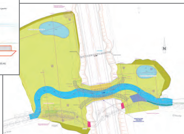
Cross-section of the Bras d'Altorf structure and ground plane of the ecological developments on the watercourse. Project study for the western bypass of Strasbourg. SOCOS/SINBIO.
