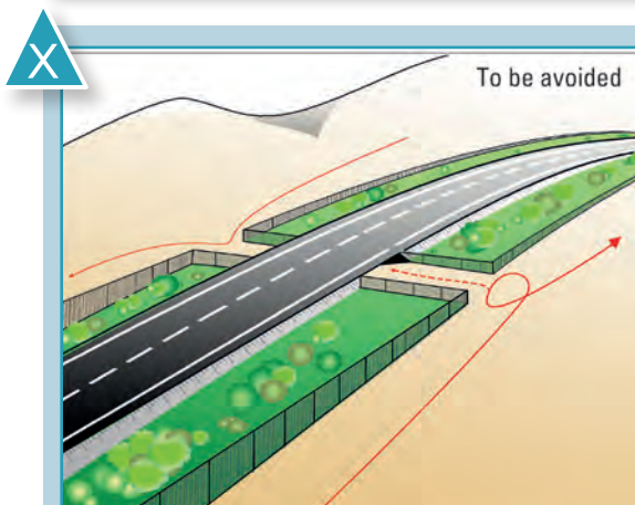
3 The layout of the fencing does not leave the green rights-of-way accessible to wildlife. Its layout near the entrance of the structure creates a corridor effect that deters wildlife. Source: Cerema.
