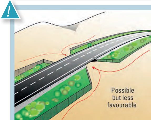
2 Layout diagram of fencing that does not leave green rights-of-way accessible to wildlife. Approaching the structure, even if the rights-of-way are not accessible, the addition of "funnel-shaped" fencing makes it possible to guide the fauna towards the entrance of the passage. Source: Cerema.
