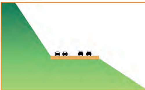
5 Schematic example of a pronounced mixed profile where the insertion of a structure is complex. Source: Cerema.
