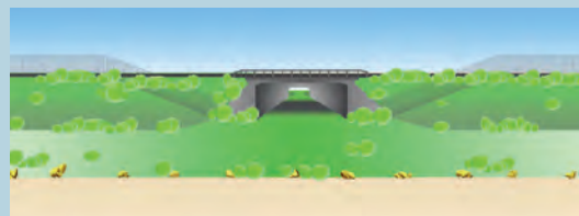
1 Layout diagram of fencing allowing wildlife to access green rights-of-way and be guided to crossing structures. Source: Cerema.
