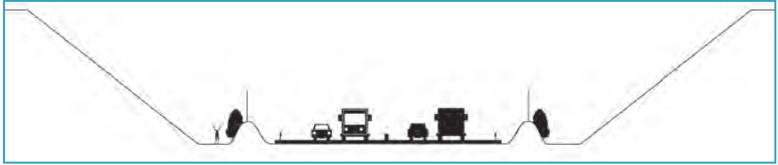
② Development plan of mounds in an excavated zone ensuring the tranquillity of rights-of-way for terrestrial fauna. Source: Cerema.
