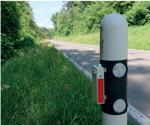
Acoustic device attached to posts and triggered by the light of an approaching vehicle.
