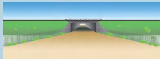
2 Layout diagram of fencing that does not leave green rights-of-way accessible to wildlife. Approaching the structure, even if the rights-of-way are not accessible, the addition of "funnel-shaped" fencing makes it possible to guide the fauna towards the entrance of the passage. Source: Cerema.
