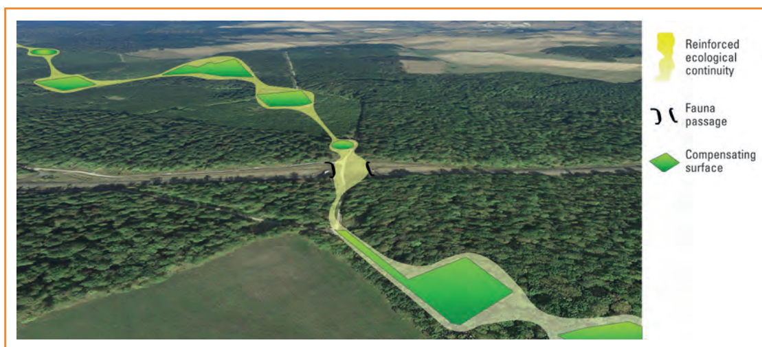
38 Schematic example of improvement of the ecological network by suitable positioning of the compensatory surfaces. Sources: Cerema, Google Earth.
