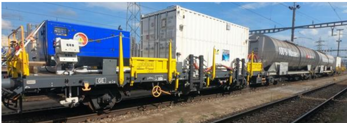
Figure 20: SBB Prototype "Hot water spot-spray train"
