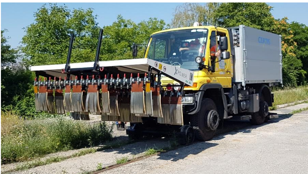
Figure 8: ÖBB-Infra - Road-rail vehicle electro-weeding Certis-Zasso University of Applied Sciences Carinthia
