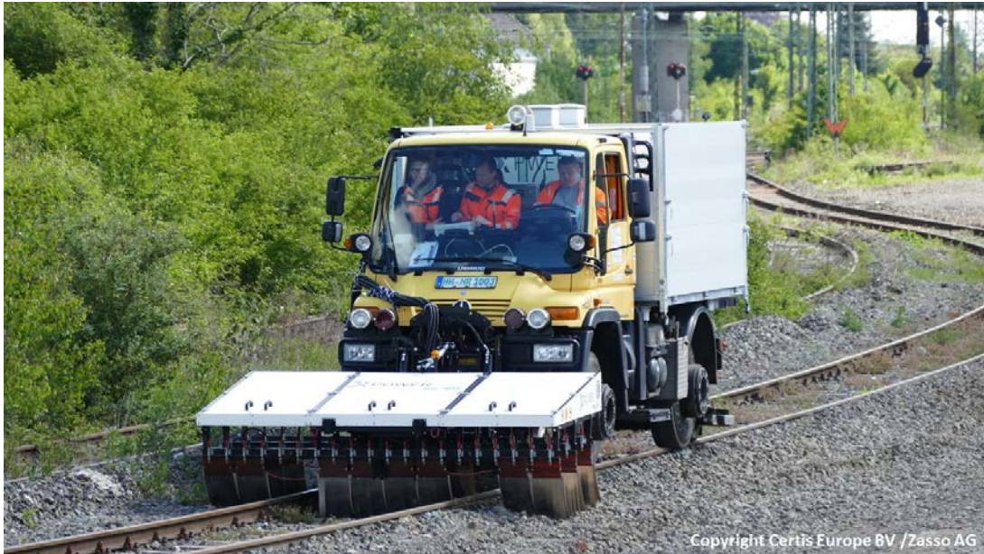
Figure 2: Pilot system for electro-weeding on a road-rail vehicle
