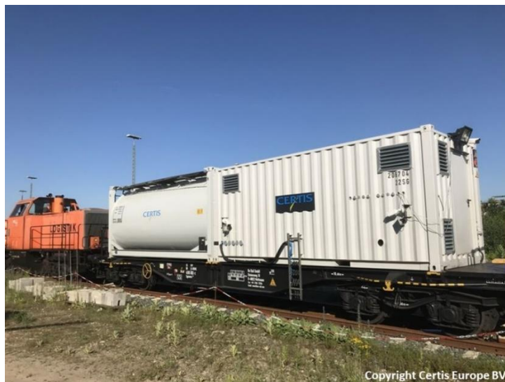
Figure 7: Modern spray train equipped with cameras for vegetation detection and GPS for taking protected areas into account
