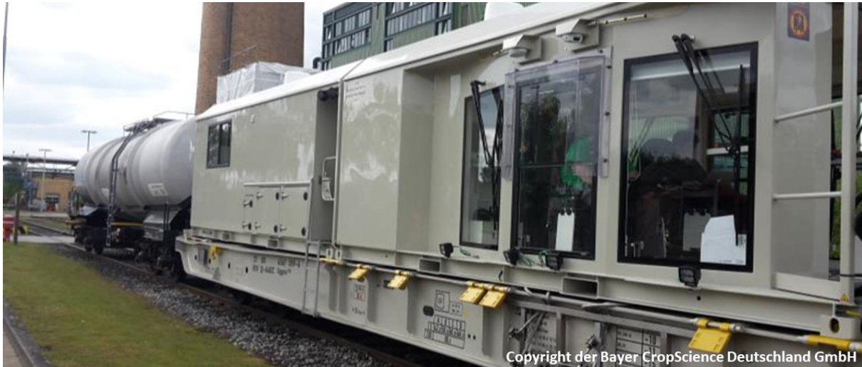
Figure 18: Modern spray train equipped with cameras for vegetation detection and GPS for taking protected areas into account
